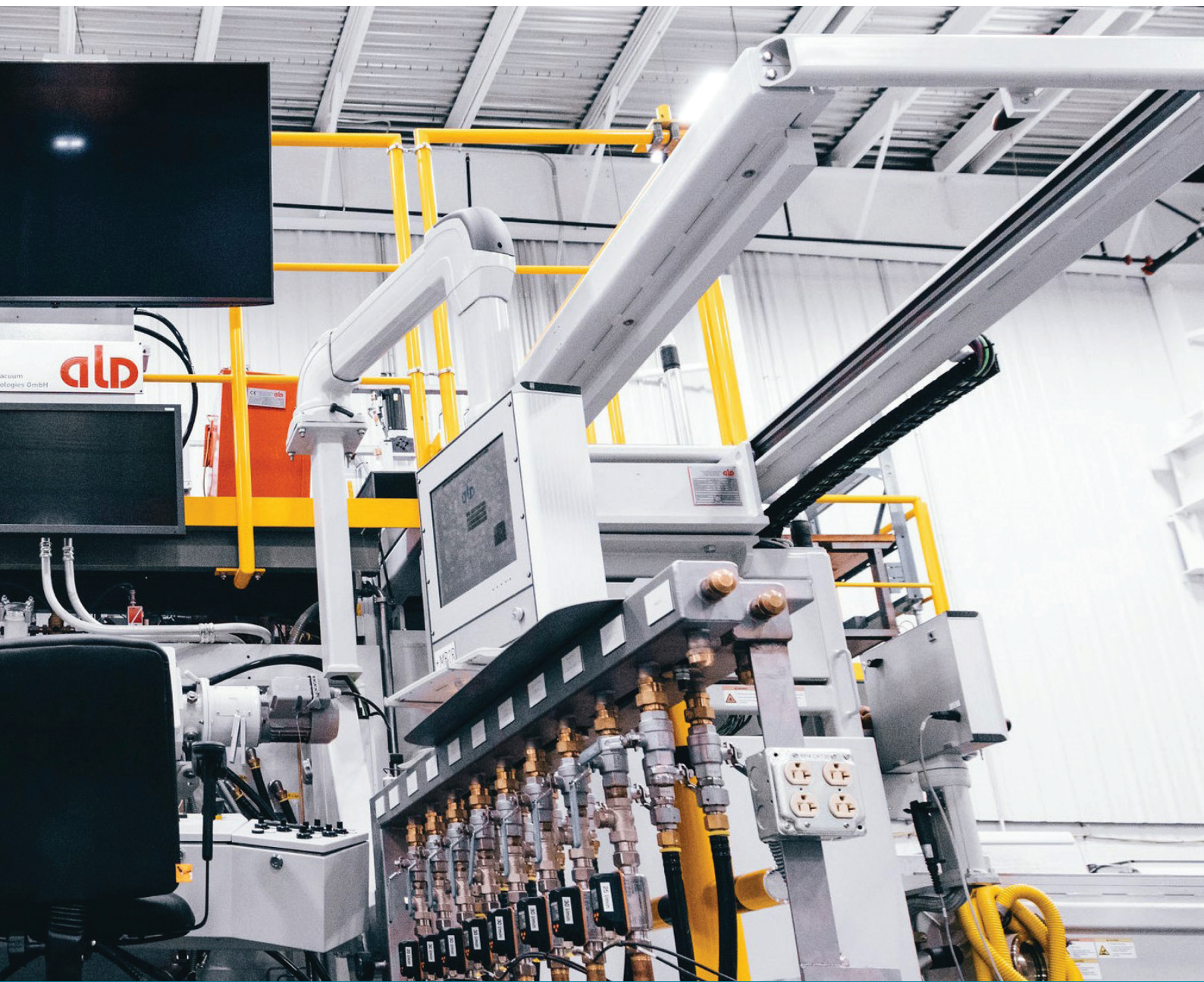
AMG Engineering coater for the production of Thermal Barrier Coatings; Source: Honeywell
